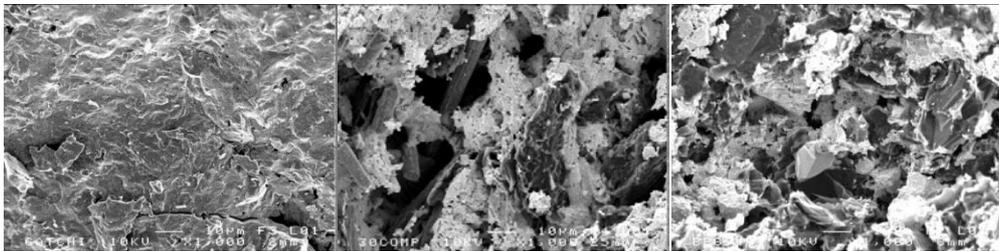
Figure 2. SEM images. From left to right: compact structure of high-density UC, open structure containing UC<sub>2</sub> grains and carbon fibers, open structure containing UC<sub>2</sub> grains and graphite residual clusters (black blocks).
