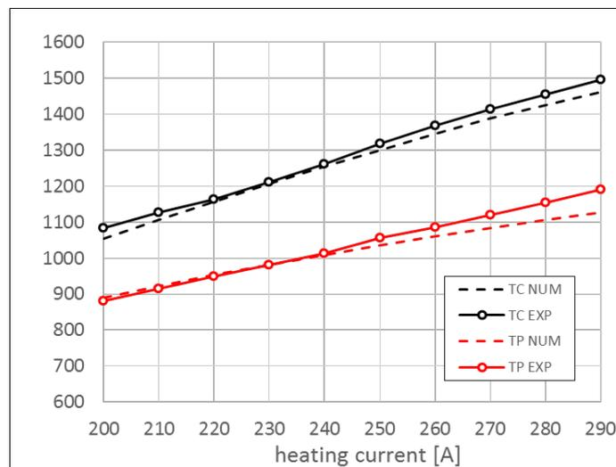
Figure 6. Experimental and numerical temperatures on center and periphery of a UC<sub>x</sub> disc.
