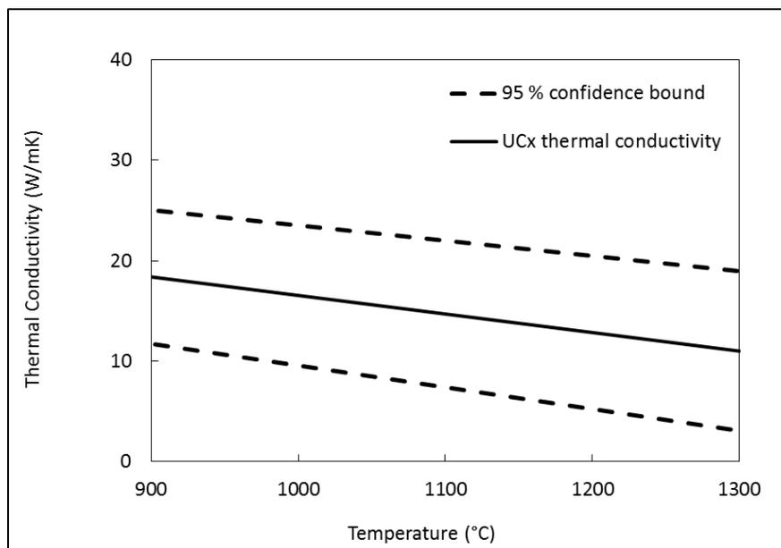
Figure 7. Thermal conductivity of UC<sub>x</sub>.
