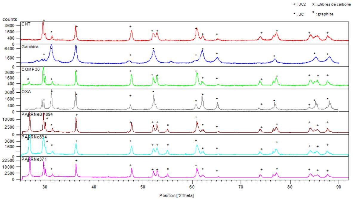
Figure 1. XRD patterns of different samples, highlighting the presence of UC, UC<sub>2</sub>, graphite and carbon microfibres.
