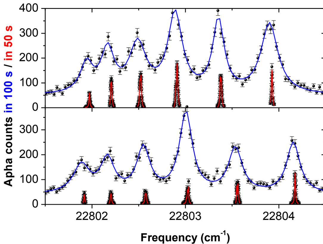
**Figure 1.** Experimental traces of the hyperfine structure in the  ${}^2D_{3/2} \rightarrow {}^4P_{5/2}$  transition at 438 nm for the actinium isotopes  ${}^{214,215}\text{Ac}$  using in-gas-cell (blue curve) and in-gas-jet (red curve).
