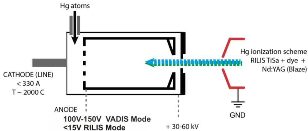
**Figure 2.** Schematic view of the laser ionization zone in VADIS.
