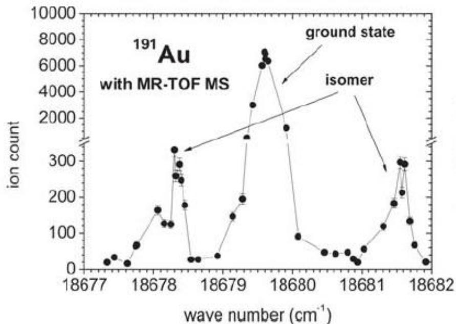
**Figure 5.** The  $^{191}\text{Au}$  ToF-gated ion-count rate at the MR-ToF detector as a function of the laser frequency of first excitation step of the Au ionization scheme.
