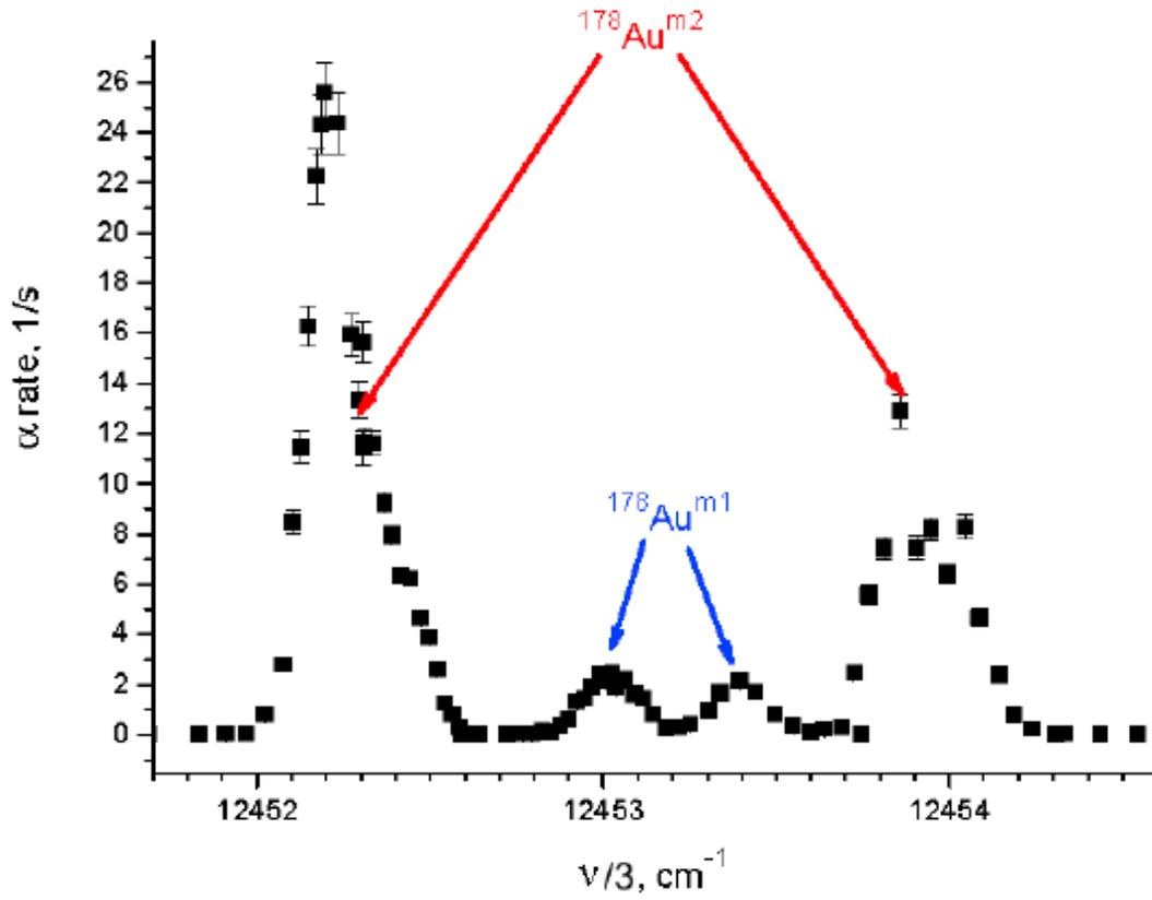
Figure 6. Hyperfine structure for  $^{178}\text{Au}$  measured with the “Windmill”  $\alpha$ -decay setup.
