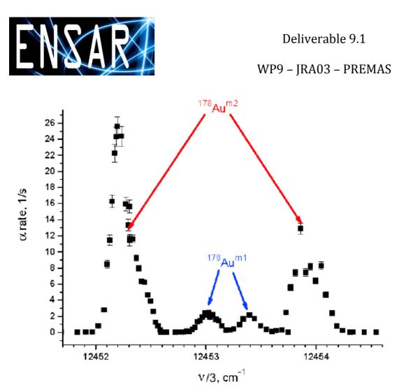
Figure 6. Hyperfine structure for  $^{178}$ Au measured with the "Windmill"  $\alpha$ -decay setup.
