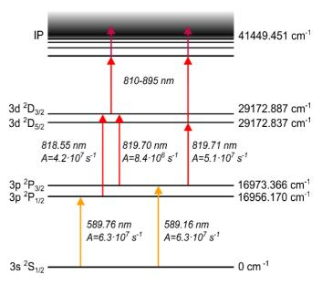
Figure 4. Three step excitation schemes in Na.
