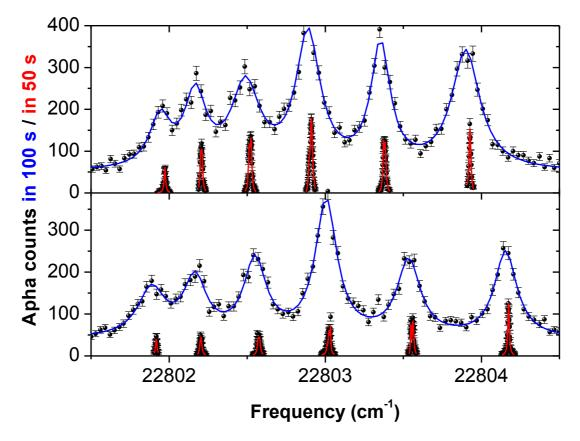
**Figure 1.** Experimental traces of the hyperfine structure in the  ${}^{2}D_{3/2} \rightarrow {}^{4}P_{5/2}$  transition at 438 nm for the actinium isotopes  ${}^{214,215}$ Ac using in-gas-cell (blue curve) and in-gas-jet (red curve).
