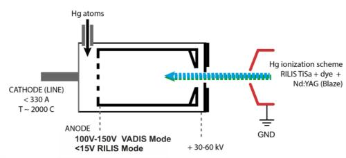
Figure 2. Schematic view of the laser ionization zone in VADIS.
