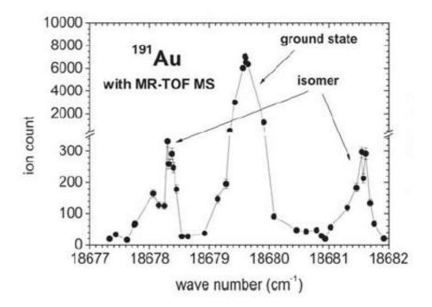
**Figure 5.** The <sup>191</sup>Au ToF- gated ion-count rate at the MR-ToF detector as a function of the laser frequency of first excitation step of the Au ionization scheme.
