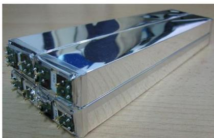
Fig 2: A set of four CsI crystals, wrapped in ESR, as would be held in a single carbon fibre alveolus. Mounted on the exit face are the accompanying Hamamatsu S12102 double APDs.
