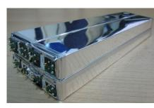
Fig 2: A set of four CsI crystals, wrapped in ESR, as would be held in a single carbon fibre alveolus. Mounted on the exit face are the accompanying Hamamatsu S12102 double APDs.
