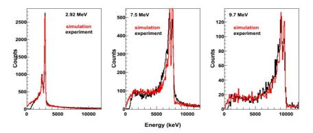
**Figure 3**: Comparison of experimental and simulation spectra for three different tagged gamma energies. High energy gamma-rays were produce in the DALINAC-NEPTUN facility and were recorded with a small prototype mounted with 14 CsI(TI)+ APDs.
