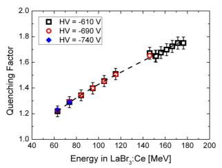
**Figure 7:** The measured quenching (preliminary data) factor measured for protons in a LaBr3:Ce 3"x3" detector. The plot have been taken from A.Giaz et al. Conference Record NP01-21 IEEE-NSS Seoul 2013.
