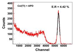
**Figure 1:** Example of the best energy resolution achieved for 1cm3 CsI(Tl)coupled to a S8664-1010 Avalanche Photo Diode (APD)
