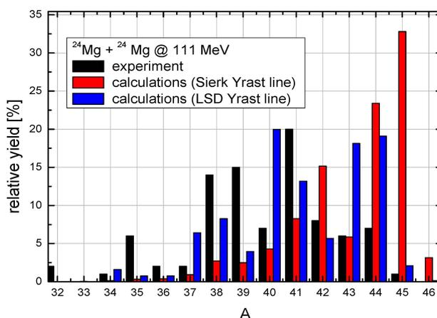
Fig.9 The evaporation residues for reactions leading to  $^{48}\text{Cr}$ . Comparison of the experimental mass distribution and GEANT4 calculations with the RLSD and FRLDM yrast line.
