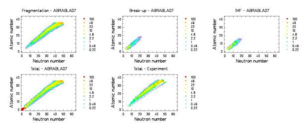
Fig. 1: Calculated and measured cross sections for the reaction <sup>86</sup>Kr(500AMeV)+Be shown on the nuclide chart. Up – different contributions to the total production cross section as predicted by ABRABLA07 (fragmentation, simultaneous break-up, intermediate-mass fragment evaporation). Down – total production cross sections: left are shown ABRABLA07 predictions, right are shown experimental data.
