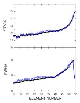
Fig. 8: Mean-neutron to proton ratio (up) and FWHM (down) of the isotopic distributions for the reaction <sup>136</sup>Xe(1000AMeV)+Pb: Experimental data (black dots), ABRABLA07 predictions: total (blue dots).
