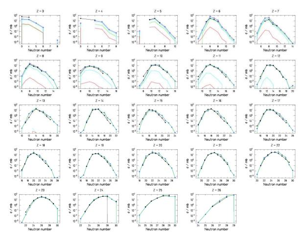
Fig. 5: Isotopic production cross sections for the reaction <sup>56</sup>Fe(1000AMeV)+Ti: Experimental data (black dots), ABRABLA07 predictions: total (blue dots), break-up (red line), IMF evaporation (light blue line), fragmentation (green line).
