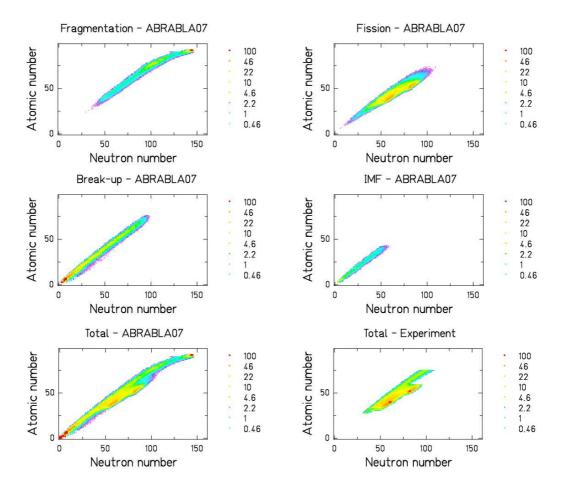
Fig. 12: Calculated and measured cross sections for the reaction <sup>238</sup>U(1000AMeV)+Pb shown on the nuclide chart. Up and middle – different contributions to the total production cross section as predicted by ABRABLA07 (fragmentation, fission, simultaneous break-up, intermediate-mass fragment evaporation). Down – total production cross sections: left are shown ABRABLA07 predictions, right are shown experimental data.
