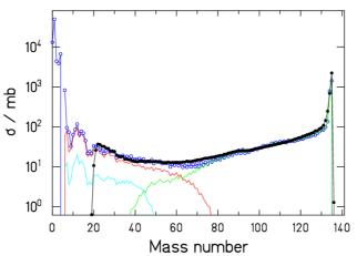
Fig. 9: Mass distribution for the reaction <sup>136</sup>Xe(1000AMeV)+Pb: Experimental data (black dots), ABRABLA07 predictions: total (blue dots), break-up (red line), IMF evaporation (light blue line), fragmentation (green line).
