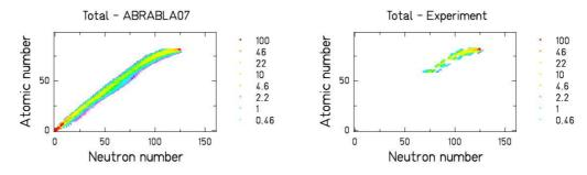
Fig. 10: Calculated and measured cross sections for the reaction <sup>208</sup>Pb(1000AMeV)+Cu shown on the nuclide chart. Up and middle – different contributions to the total production cross section as predicted by ABRABLA07 (fragmentation, fission, simultaneous break-up, intermediate-mass fragment evaporation). Down – total production cross sections: left are shown ABRABLA07 predictions, right are shown experimental data.
