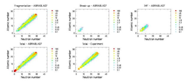
Fig. 4: Calculated and measured cross sections for the reaction  ${}^{56}Fe(1000AMeV)$ +Ti shown on the nuclide chart. Up – different contributions to the total production cross section as predicted by ABRABLA07 (fragmentation, simultaneous break-up, intermediate-mass fragment evaporation). Down – total production cross sections: left are shown ABRABLA07 predictions, right are shown experimental data.
