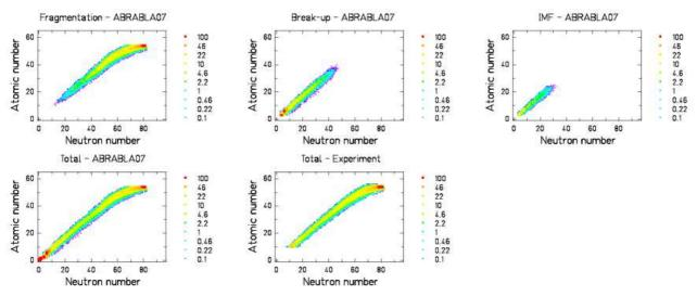
Fig. 7: Calculated and measured cross sections for the reaction <sup>136</sup>Xe(1000AMeV)+Pb shown on the nuclide chart. Up – different contributions to the total production cross section as predicted by ABRABLA07 (fragmentation, simultaneous break-up, intermediate-mass fragment evaporation). Down- total production cross sections: left are shown ABRABLA07 predictions, right are shown experimental data.
