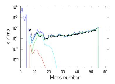
Fig. 6: Mass distribution for the reaction <sup>56</sup>Fe(1000AMeV)+Ti: Experimental data (black dots), ABRABLA07 predictions: total (blue dots), break-up (red line), IMF evaporation (light blue line), fragmentation (green line).
