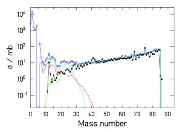
Fig. 3: Mass distribution for the reaction <sup>86</sup>Kr(500AMeV)+Be: Experimental data (black dots), ABRABLA07 predictions: total (blue dots), break-up (red line), IMF evaporation (light blue line), fragmentation (green line).
