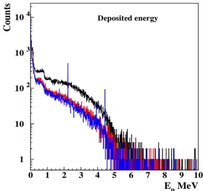
Fig. 8. The black curve shows the deposited energy spectrum in the NaI crystal. The energy of incoming neutrons is 5 MeV. A 10 cm long water tube or 10 cm long paraffin tube was placed as a shielding just in front of the crystal. The red curve indicates the effect of the water; the blue curve shows the effect of the paraffin shield. There is no significant difference between the effect of the paraffin and water shield.
