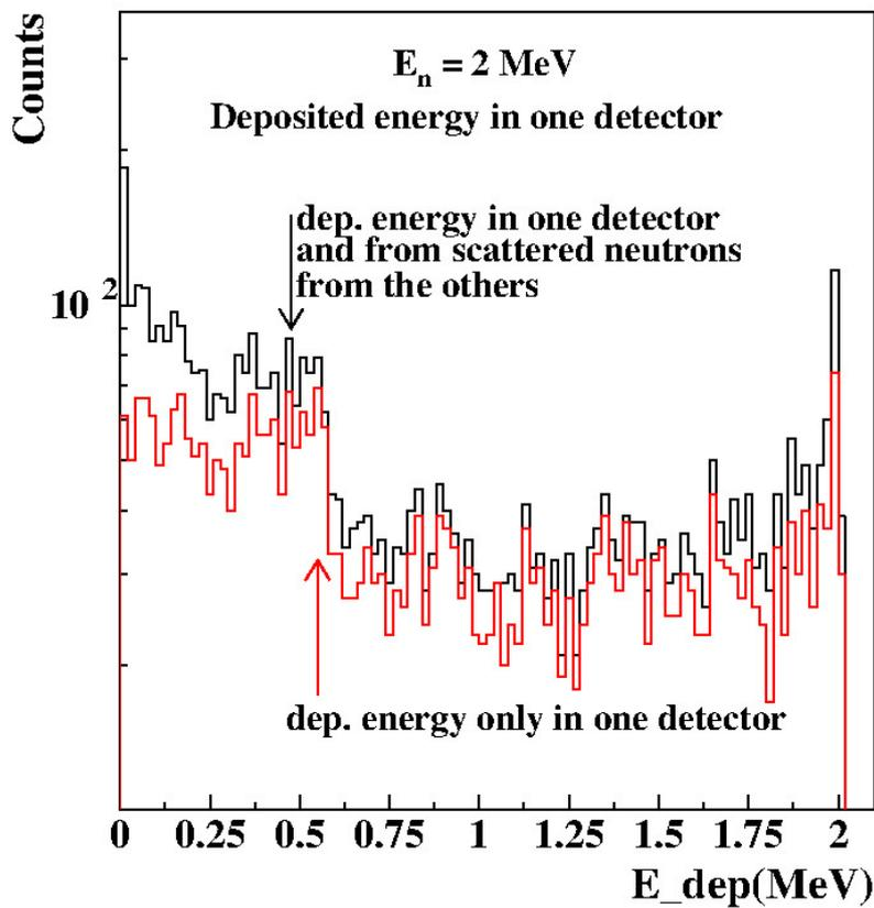
Fig. 5 Study of cross-talk between the bars. Red line indicates the deposited energy in one scintillator bar with the condition that no other detector bars fired. Black line shows the deposited energy in one bar without any condition.
