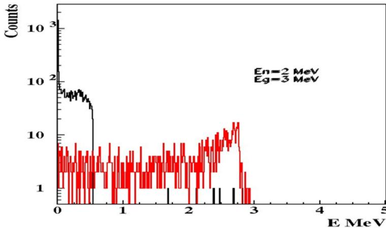
Fig. 6. The simulated response functions for 2 MeV neutrons (black histogram) and for 3 MeV gamma rays (red histogram) as a function of electron-equivalent energy.
