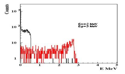
Fig. 6. The simulated response functions for 2 MeV neutrons (black histogram) and for 3 MeV gamma rays (red histogram) as a function of electron-equivalent energy.
