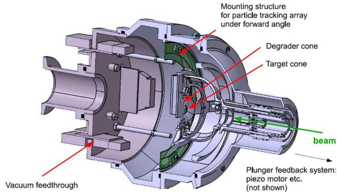
FIG. 4: Sectional view of a plunger endcap with tracking capabilities for low-energy beams (see text). Not shown is the mechanics of the plunger feedback system.
