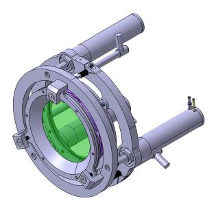
FIG. 5: Schematic drawing of the HISPEC plunger device. Near to each of the three linear actuators an inductive sensor is mounted which is clearly visible close to the upper actuator to measure independently the movements induced by the actuator.
