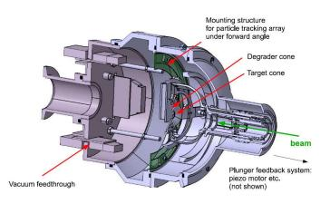
FIG. 4: Sectional view of a plunger endcap with tracking capabilities for low-energy beams (see text). Not shown is the mechanics of the plunger feedback system.
