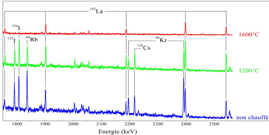
**Fig.9:** Release properties of various prototypes of  $\text{UC}_x$  pellets at 1600 °C (courtesy of E. Cottureau et al., proceedings of Eurisol-Net meeting at CERN, June 27-28, 2011)
