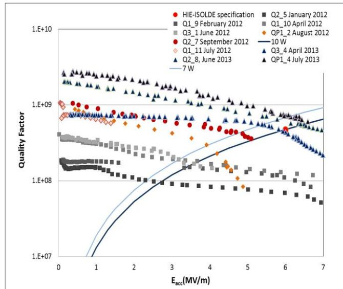
**Fig.11:** Q vs.  $E_{acc}$  curves of bias diode coated cavities [23]
