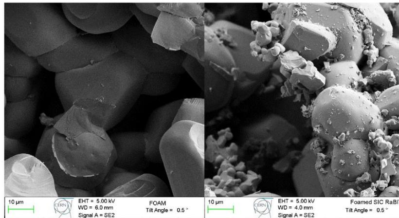
**Fig.5:** SEM analysis of the samples irradiated with RaBIT at 5000x before (left) and after irradiation (right) [10]
