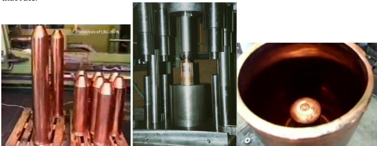
The laboratory is also investigating three other fabrication methods: forward flow-turning, and both direct and reverse deep-drawing [26].
