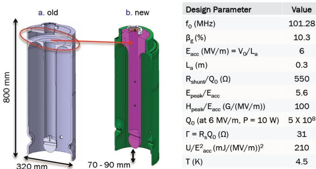
**Fig.10:** HIE-ISOLDE high-beta Copper substrates: left) rolled and welded prototype; right) bulk machined prototype (inner conductor shown in magenta);
