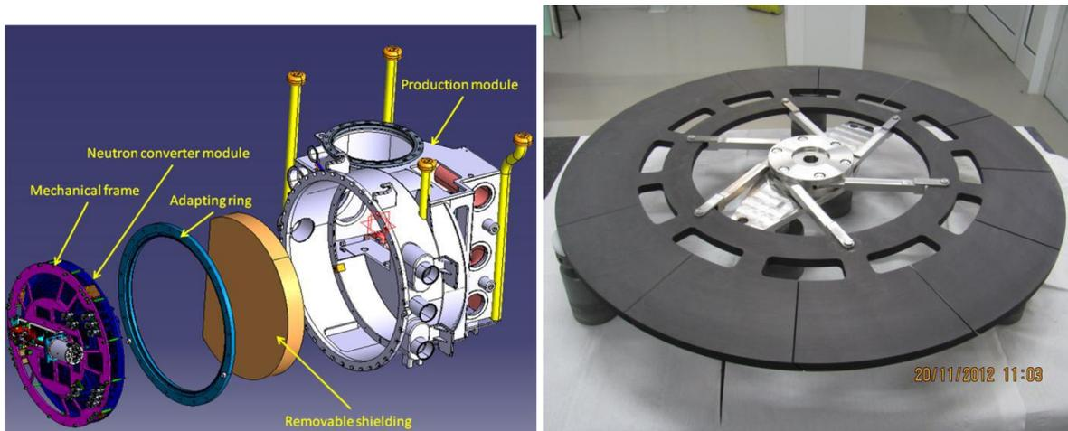
**Fig.2:** 3D View of the neutron converter and a picture of the 50 kW graphite prototype target
