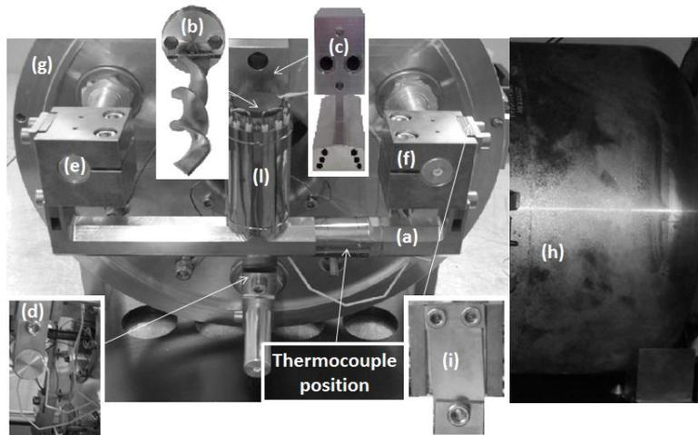
**Fig.6:** NaF:LiF Molten Salt Target unit before irradiation [11]: (a) Container; (b) Helical Transfer Line; (c) Cold Line; (d) Ion Source; (e) Feed through; (f) Connection Block; (g) Flange; (h) Vessel; (i) Electrical Connection; (l) Screen.
