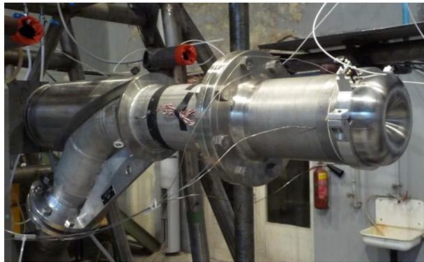
**Fig.1:** EURISOL liquid metal neutron converter target on test stand at IPUL
