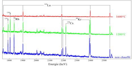
**Fig.9**: Release properties of various prototypes of UC<sub>x</sub> pellets at 1600 °C (courtesy of E. Cottereau et al., proceedings of Eurisol-Net meeting at CERN, June 27-28, 2011)
