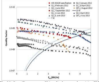
Fig.11: Q vs. Eacc curves of bias diode coated cavities [23]
