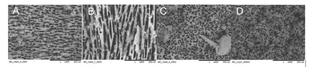
**Fig.4:** SEM images of ice-templates green bodies of the same powder sub- ject to different parameters modifications listed in Table 1: (A) fast-freezing; (B) slow-freezing; (C) addition of ZRA - honeycomb-like structure; (D) over- loaded slurry [9].
