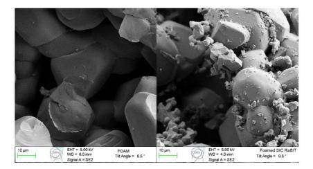
**Fig.5:** SEM analysis of the samples irradiatied with RaBIT at 5000x before (left) and after irradiation (right) [10]
