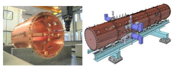
Fig.12a: SPIRAL 2 RFQ prototype cavity[25] Fig.12b: Artistic view of the final SPIRAL2 RFQ [25]
