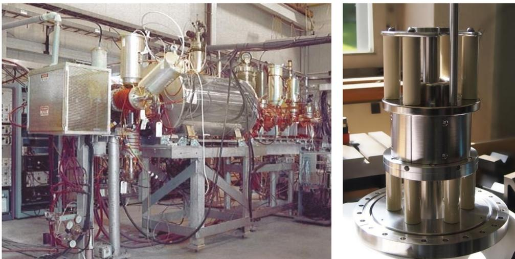
**Figure 1 Left: BNL EBCB test stand. Suitable for HEC2 tests and operational. Right: HEC2 electron gun pre-assembled at CERN.**
