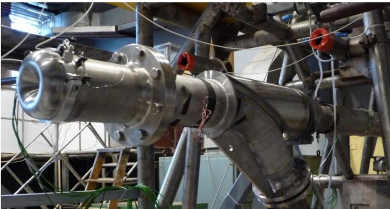
Figure 1: EURISOL Liquid metal neutron converter on test stand at IPUL
