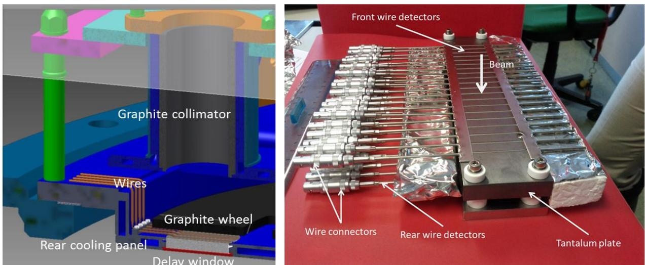
**Figure 6.** A sketch of the Delay Window (left) and the prototype tested with e-beam (right).
