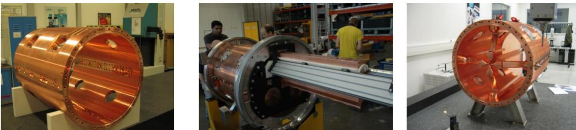
**Figure 8.** From left to right: a copper tube, inserting an electrode in a tube, a completed module.
