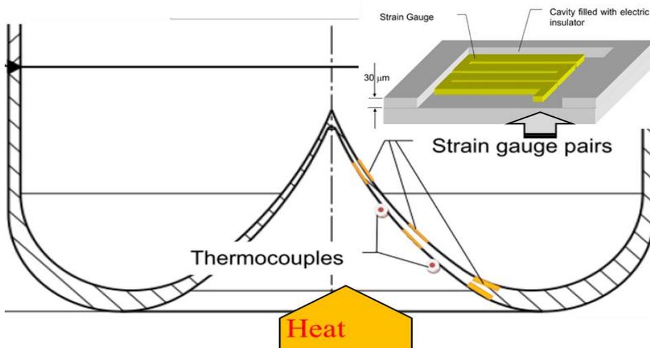
Figure 3: Schematic of beam setup on beam window
