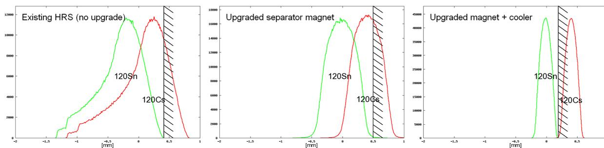
**Figure 6: Example calculated beam profiles of the HRS**
