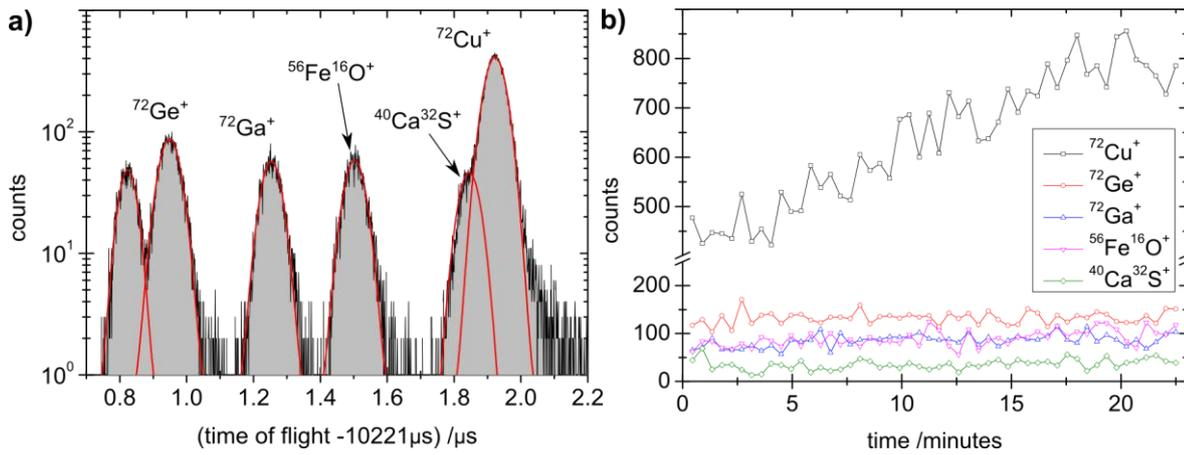
Fig. 2: a) Integral time-of-flight spectrum for  $A = 72$  as delivered from ISOLDE during heating of the target material; b) Number of counts of the isotopes from the spectrum on the left as a function of the time and increase of the target heating by approximately  $70^\circ\text{C}$  [9].
