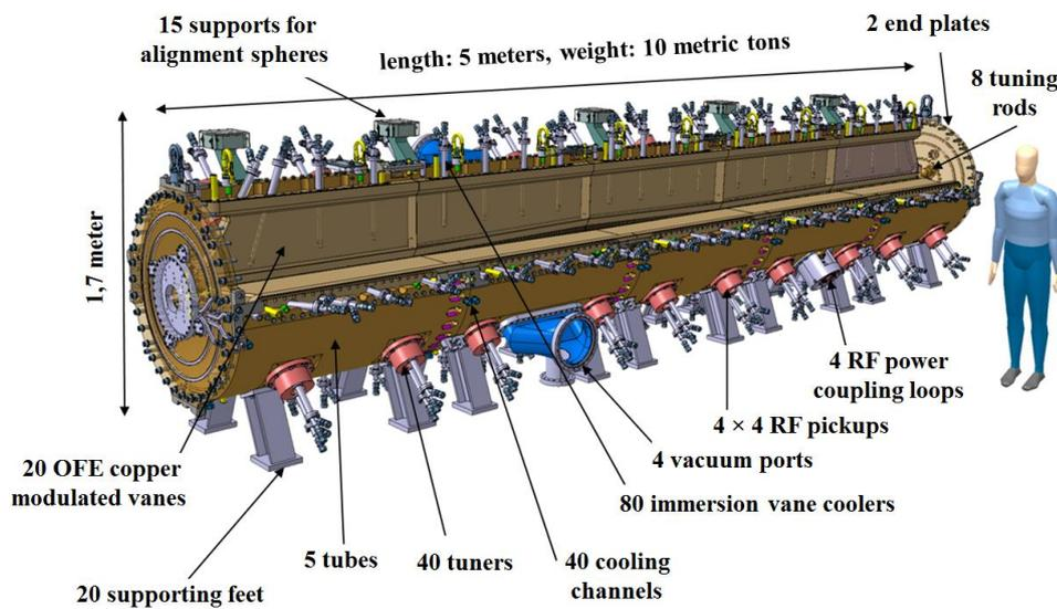
**Figure 7.** The SPIRAL2 RFQ (tube is opened along one quadrant).
