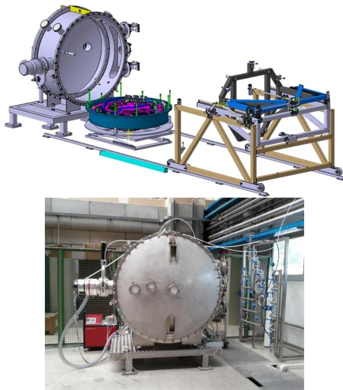
**Figure 7.** A sketch of the of the maintenance tool (left) and a picture of the production module housing the neutron converter module(right) .
