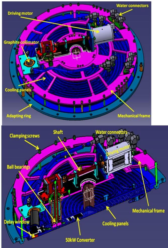
**Figure 2.** Left – A general view of the NCM. Right – a transversal cut of the NCM showing the internal components
