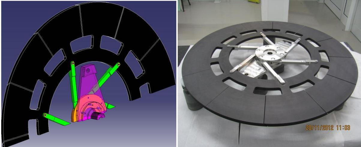
**Figure 3.** A conceptual sketch of the graphite wheel and a picture of the 50kW prototype.
