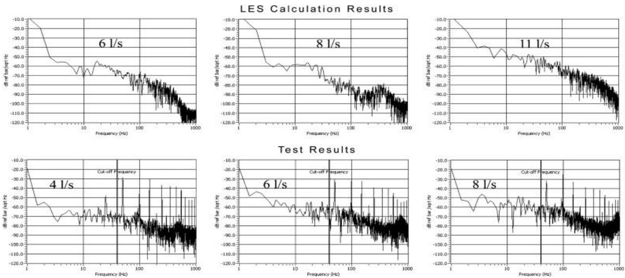
Figure 2: Comparison of pressure fluctuation spectral densities calculated (top) and measured (bottom) in the hydraulic test
