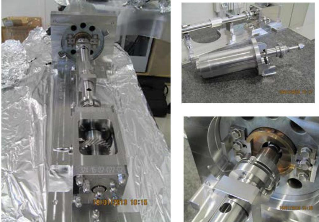
**Figure 4.** Rotation system for the 50 kW converter. The system has been conceived to replace the block with bearings keeping the converter in place.
