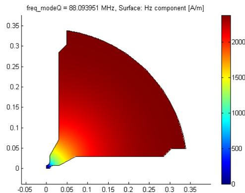
Figure 2. Magnetic field in RFQ cross-section.
