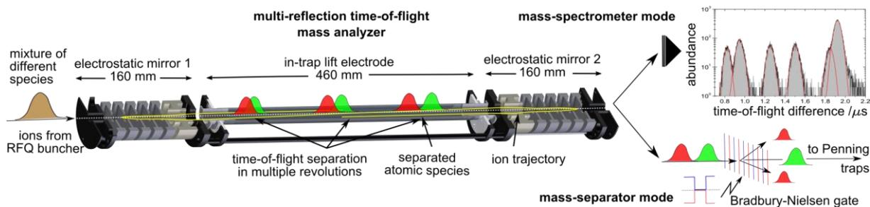
Fig. 1: Sketch of the operation principle of the ISOLTRAP MR-ToF MS as a mass analyzer and precision spectrometer in combination with an ion detector (top right) and as a mass separator in combination with a Bradbury-Nielsen beam gate (bottom right) [9].
