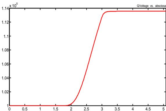
Figure 1. Inter-vane voltage (V) vs. abscissa (m).
