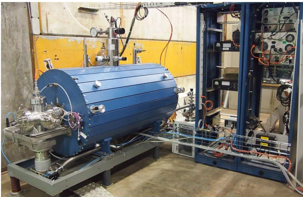
**Figure 4. TWINEBIS is a replica of REXEBIS at CERN suitable as a test stand for the debunching trap and a test stand for intermediate upgrades of REX-like breeders. Presently getting operational after relocation from Manne Siegbahn Laboratory (Stockholm) to CERN.**
