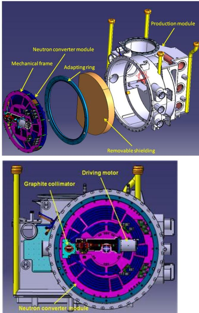
**Figure 1.** View of the neutron converter integrated inside the production module.
