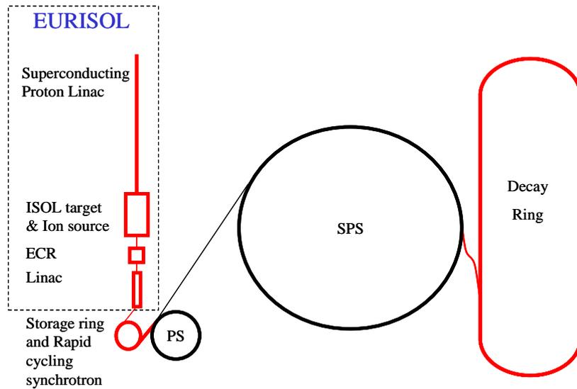
**Figure 2: Schematic view of the beta-beam facility**
