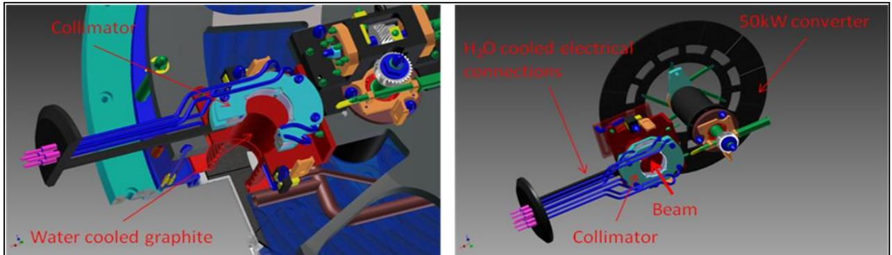
**Figure 5.** The production module with installed the beam collimator (left) and the set up for the 50 kW converter including the water cooled graphite tube (right).
