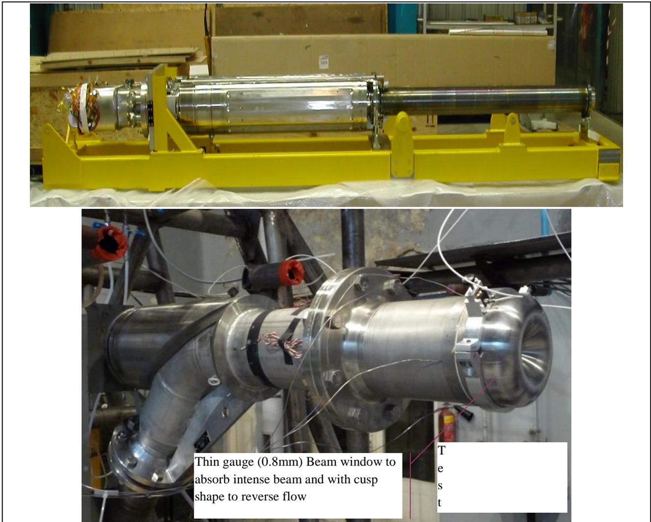
**Figure 4: Liquid metal neutron source Megapie (top), Eurisol on test stand (bottom)**
