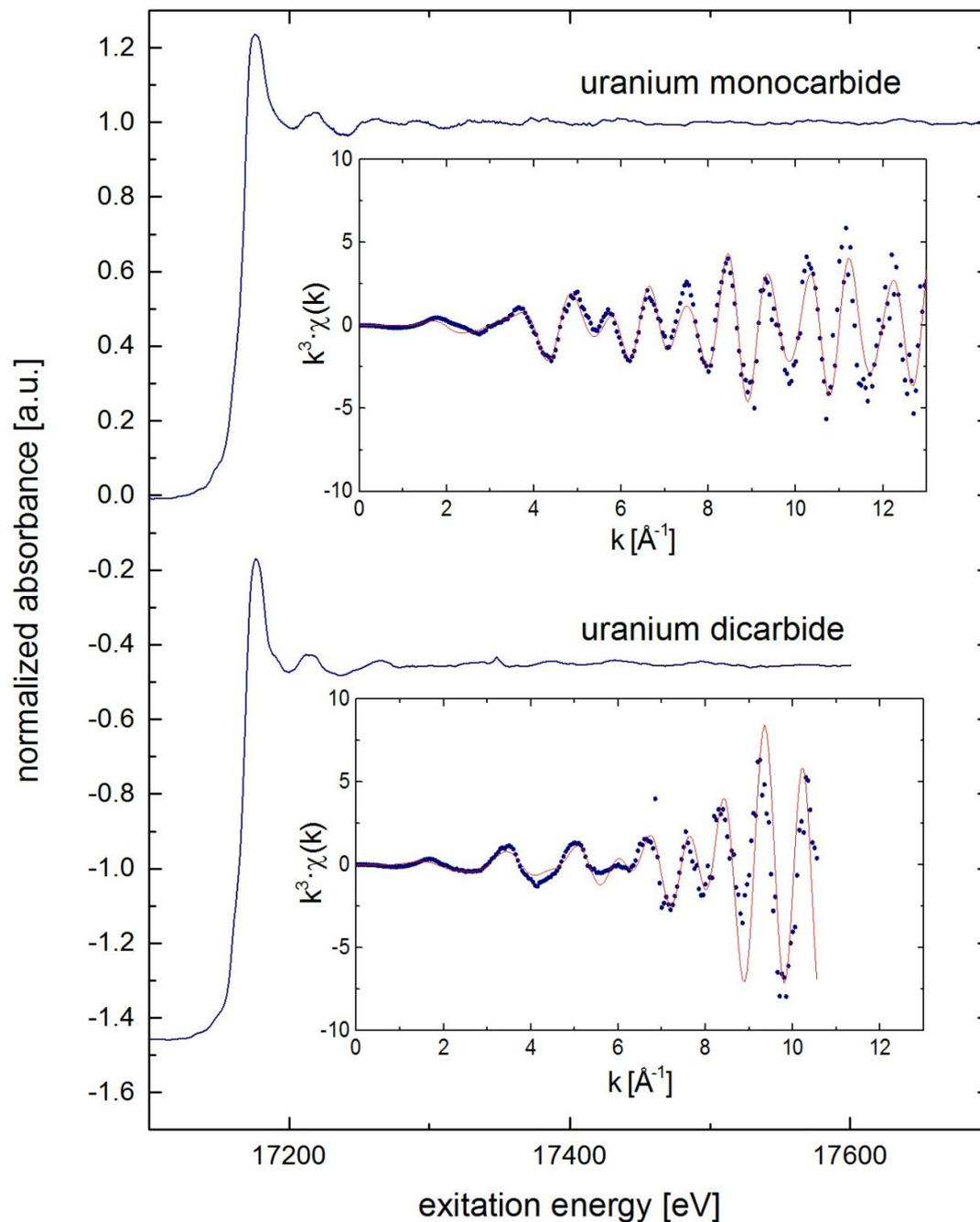
Figure 2. EXAFS spectra of uranium monocarbide measured with a  $3\mu\text{m}^2$  synchrotron focus (top) and uranium dicarbide measured with a  $1.4\mu\text{m}^2$  synchrotron focus (bottom).  $k^3$ -weighted absorbance as inset respectively (blue dots – data, red line – IFEFFIT fit for the respective structure as described in the text).
