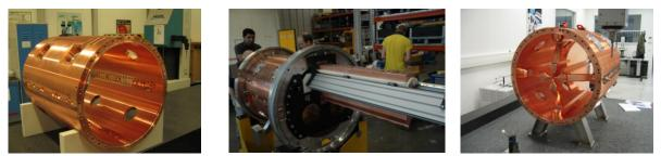
Figure 8. From left to right: a copper tube, inserting an electrode in a tube, a completed module.
