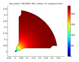
Figure 2. Magnetic field in RFQ cross-section.
