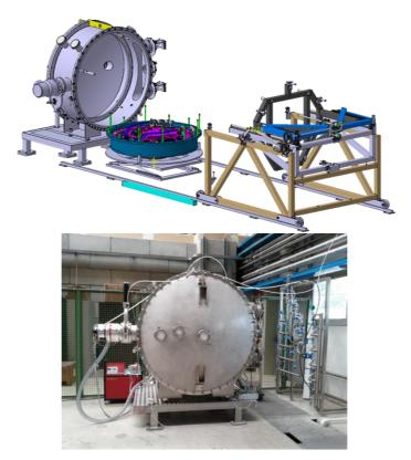
**Figure 7.** A sketch of the of the maintenance tool (left) and a picture of the production module housing the neutron converter module(right).
