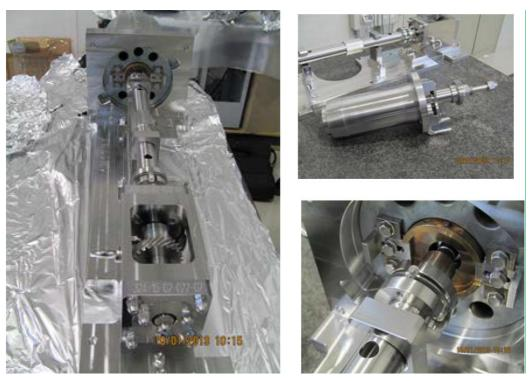
Figure 4.Rotation system for the 50 kW converter. The system has been conceived to replace<br/>the block with bearings keeping the converter in place.
