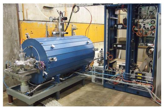
Figure 4. TWINEBIS is a replica of REXEBIS at CERN suitable as a test stand for the debunching trap and a test stand for intermediate upgrades of REX-like breeders. Presently getting operational after relocation from Manne Siegbahn Laboratory (Stockholm) to CERN.
