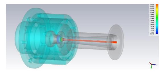
Figure 3. First test of full 3D space-charge limited electron beam with 49 keV energy and 10 A current using the CST software. The model is being integrated at CERN into CAD design workflow, has 2.74 M nodes, and the beam is created by 6170 individual trajectories. The simulation covers all aspects from emission to guiding magnetic field.
