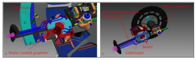
**Figure 5.** The production module with installed the beam collimator (left) and the set up for the 50 kW converter including the water cooled graphite tube (right).
