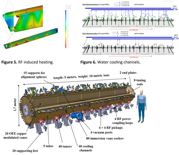
Figure 7. The SPIRAL2 RFQ (tube is opened along one quadrant).
