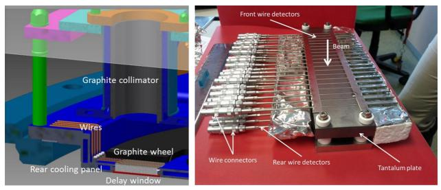
Figure 6. A sketch of the Delay Window (left) and the prototype tested with e-beam (right).
