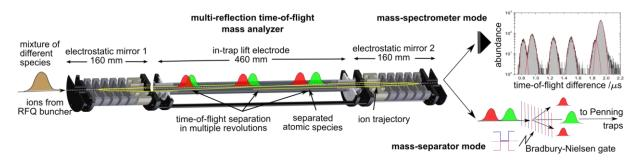
Fig. 1: Sketch of the operation principle of the ISOLTRAP MR-ToF MS as a mass analyzer and precision spectrometer in combination with an ion detector (top right) and as a mass separator in combination with a Bradbury-Nielsen beam gate (bottom right) [9].
