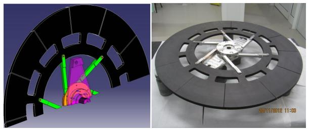
Figure 3. A conceptual sketch of the graphite wheel and a picture of the 50kW prototype.
