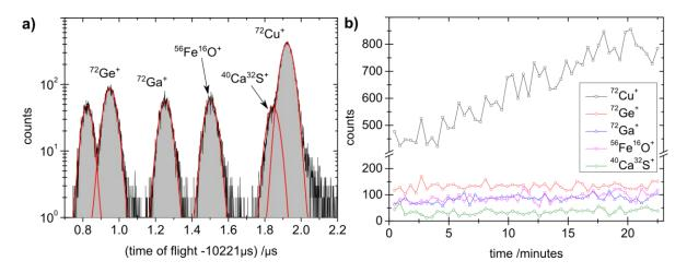
Fig. 2: a) Integral time-of-flight spectrum for A = 72 as delivered from ISOLDE during heating of the target material; b) Number of counts of the isotopes from the spectrum on the left as a function of the time and increase of the target heating by approximately 70°C [9].
