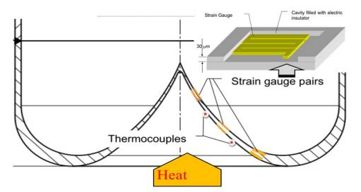
Figure 3: Schematic of beam setup on beam window
