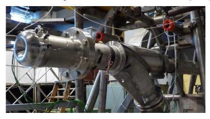
Figure 1: EURISOL Liquid metal neutron converter on test stand an IPUL
