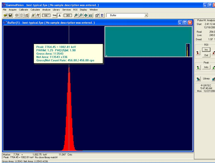
Fig. 3: Energy spectrum recorded with a pulser corresponding to a gamma-ray equivalent energy of 1 MeV.
