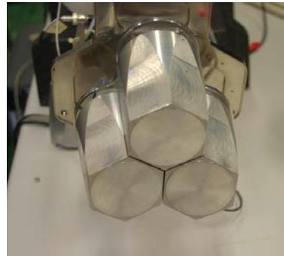
Fig. 1: The GTC cryostat fitted with the front – electronics and three dummy capsules.
