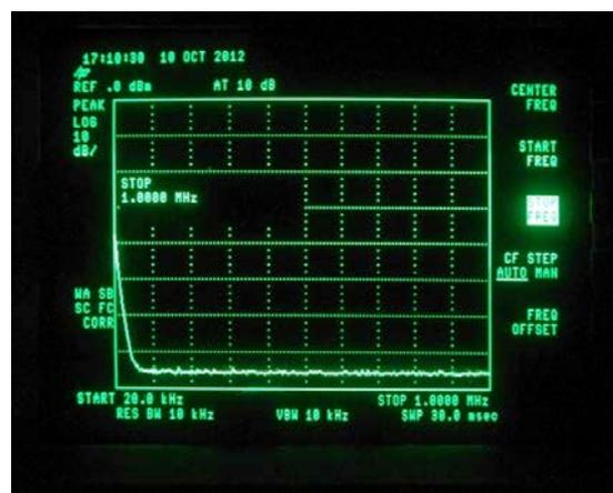
Fig. 4: Frequency spectra recorded with an HP spectrum analyzer connected at the output of the preamplifier.
