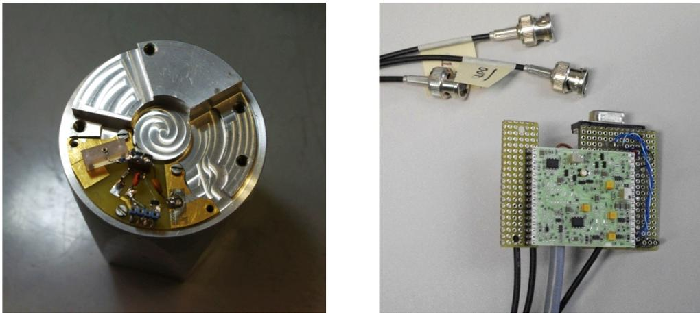
Fig. 2: The GTC cryostat fitted with the front – electronics and three dummy capsules.
