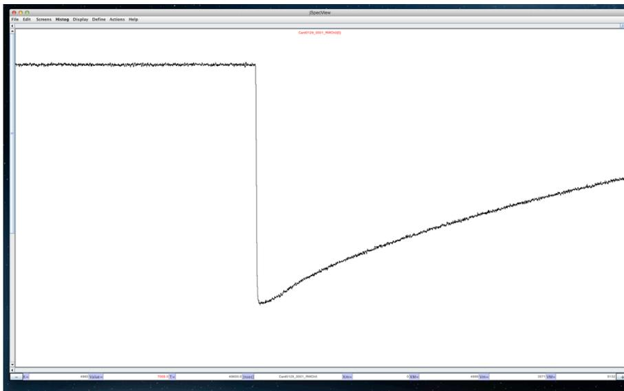
Fig. 5: Digital sampling of the pulser signal at 100 MS/s and 14 bit. The full length of the trace is 50 microsec.
