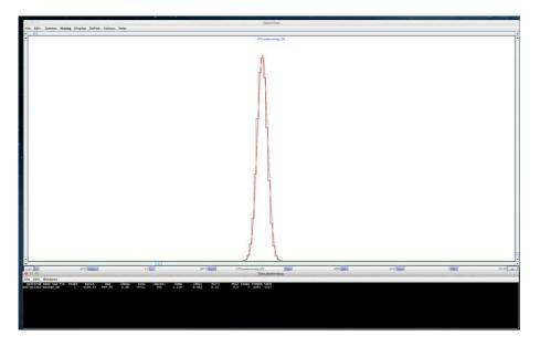
Fig. 6: Pulser peak obtained from the digital data by applying the MWD algorithm.
