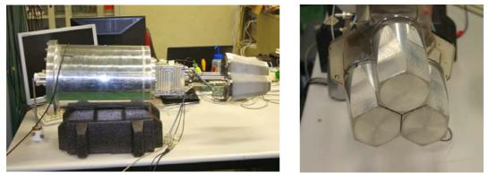
Fig. 1: The GTC cryostat fitted with the front – electronics and three dummy capsules.
