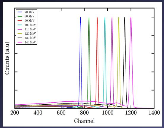
Spectra of protons at different beam energies measured with a 2" x 2"  $\times$  2" LaBr<sub>3</sub>:Ce crystal at 5 deg. relatively to the beam axis. The spectra are normalized to have the same height of a proton peak.
