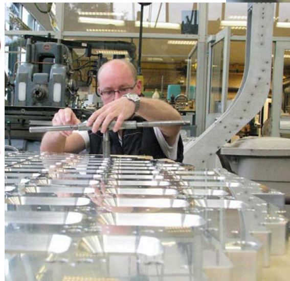
antiProton ANnihilations at Darmstadt (PANDA) Holdingstructure for calorimeter endcap
