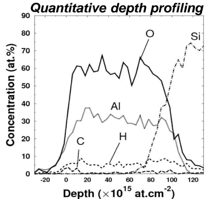
8.6 nm thick atomic layer deposited insulating  $\text{Al}_2\text{O}_3$  film on Si
